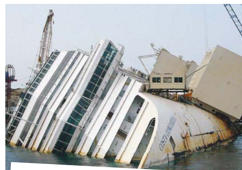
The ship was righted in September 2013 following an extremely delicate procedure known as parbuckling
