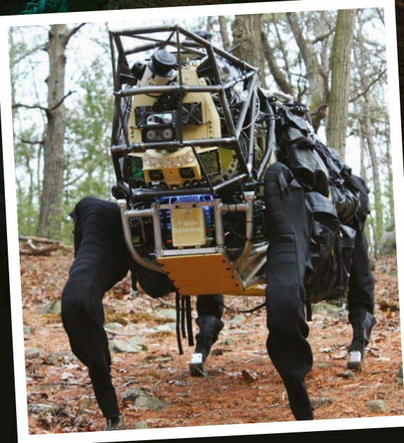
DARPA's Legged Squad Support System was designed to act as a robotic pack mule
